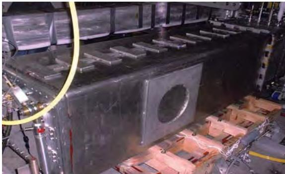
**Figure 20 Completed Maglev-2000 Quadrupole Enclosed in Cryostat**
