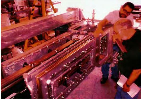
**Figure 19 Assembly of Maglev-2000 Superconducting Quadrupole**
