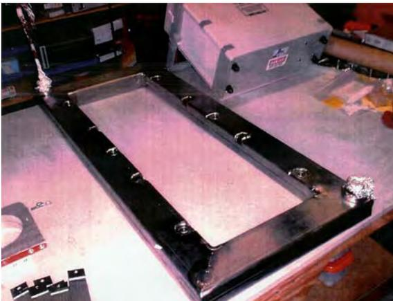
**Figure 17 NbTi Superconducting Loop Enclosed in Stainless Steel Jacket**
