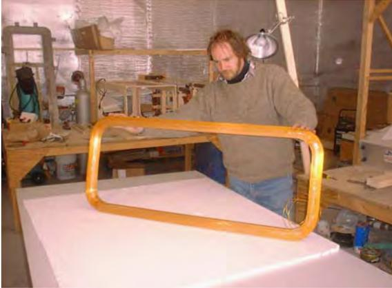
**Figure 16 NbTi Superconductor Loop for Maglev-2000 Quadrupole**
