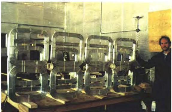
**Figure 21 Completed Guideway Panel with Figure of 8 Dipole and LSM Propulsion Loops**
