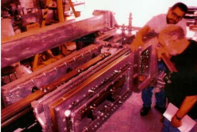
Figure 11 Assembly of Maglev-2000 Superconducting Quadrupole
