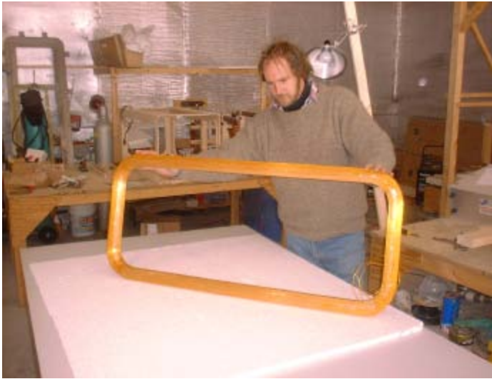
Figure 8. NbTi Superconductor Loop for Maglev-2000 Quadrupole
