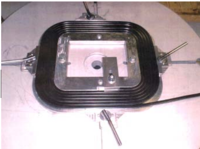
Figure 14. Wound Dipole Loop for Guideway Panel Using Nylon Coated Aluminum Conductor
