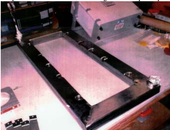
Figure 9. NbTi Superconducting Loop Enclosed in Stainless Steel Jacket
