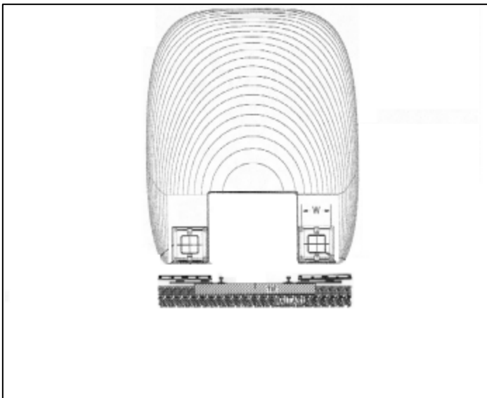
Figure 4 Drawing of Levitated maglev-2000 Vehicle Traveling on Conventional RR Tracks to Which Aluminum Loop Panels Have Been Attached to the Cross-Ties
